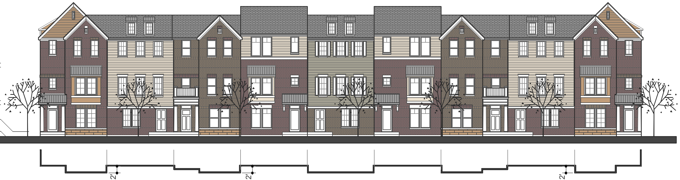
○ FRONT ELEVATION - BUILDING A (similar for all other front units on buildings B,C,D,E,F,G,H) SCALE: 1/16" = 1'-0"
