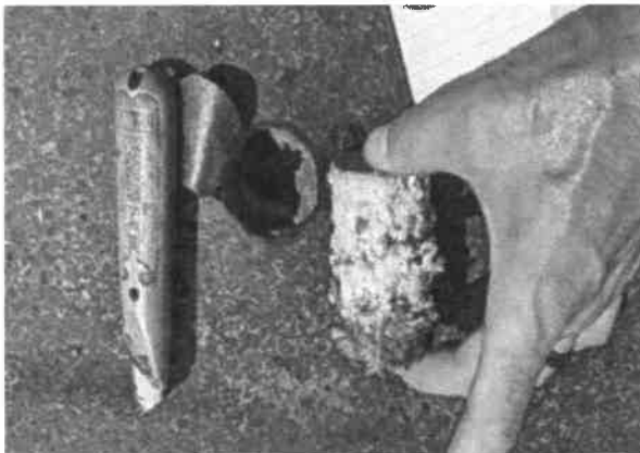
Core sample- 2.5" iso .5 wood fiber
