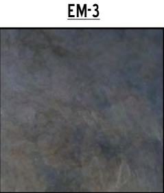
EM-3 CARBON GRADE FINISH: HOT ROLLED STEEL W/ CARBON GRADE FINISH - W/ CLEAR, MATTE POWDER COAT FINISH
