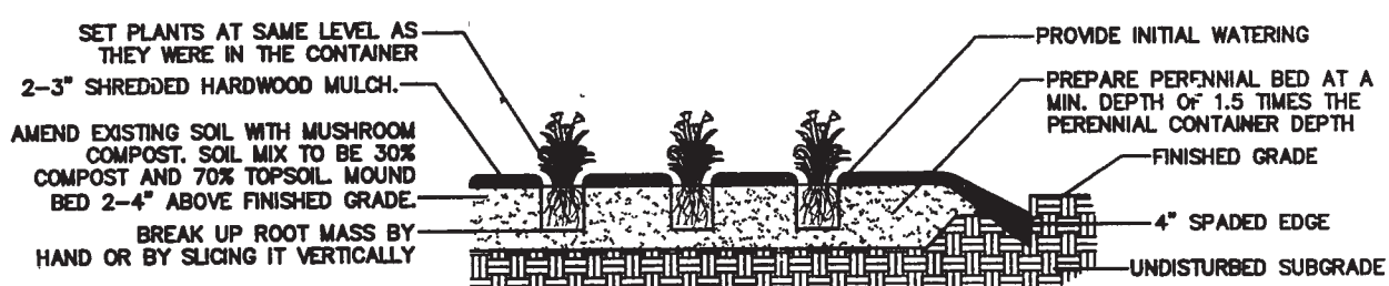
PERENNIAL PLANTING DETAIL NOT TO SCALE. USE ONLY ZONE HARDY PLANT MATERIAL.
