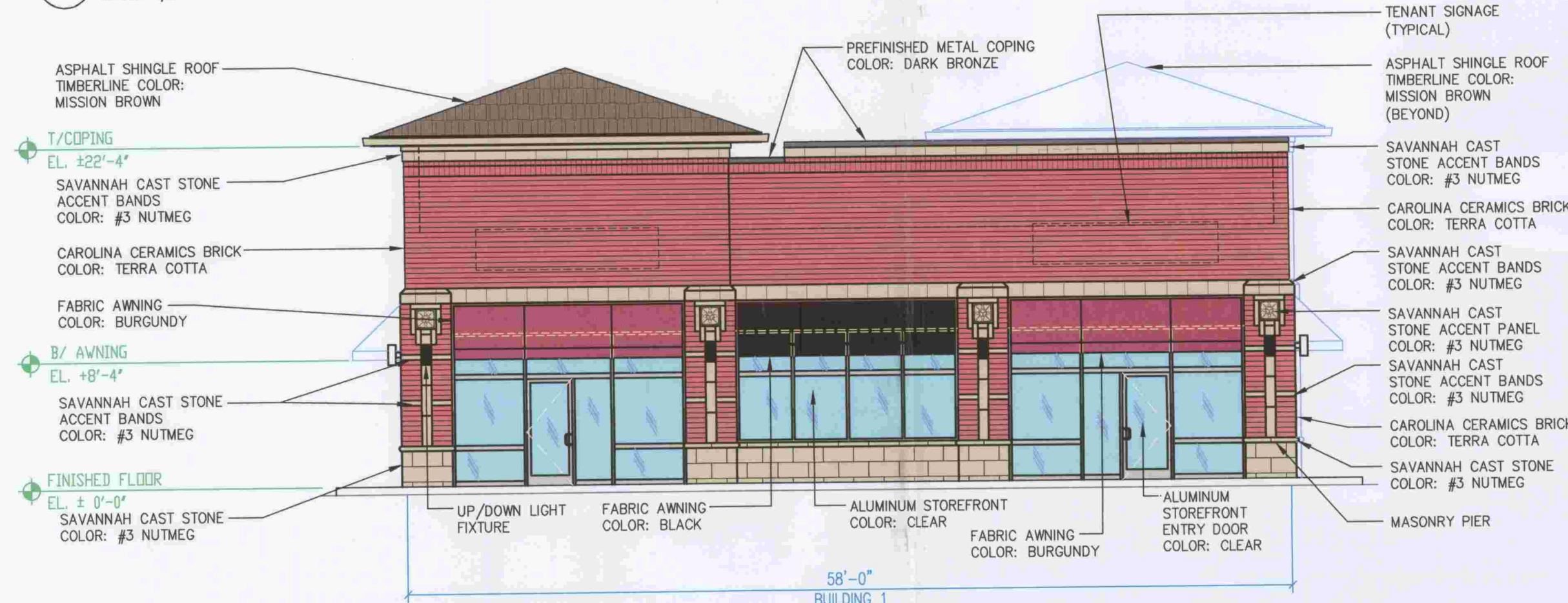
2 BUILDING 1 - EAST WALL ELEVATION
