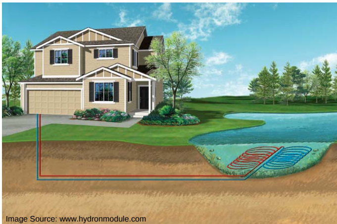
Left: Renderings that show residential and non-residential applications of hydrothermal heat pump systems using detention ponds. Above: Pond loop coils prior to being submerged into a pond. Orland Park has many residential and non-residential detention ponds that can be used as heat sources and sinks for improved energy efficiency.
