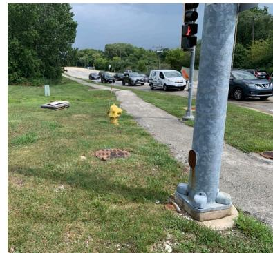
Our field investigation indicates the existing water main and fire hydrants (shown in blue line) may be in conflict with the roadway, dryland bridge, and/or storm sewer requiring relocation.
