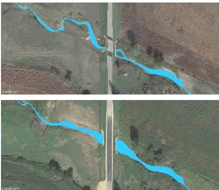
Before and after aerials of Kent Road culvert – natural stream migration after culvert location was shifted.
