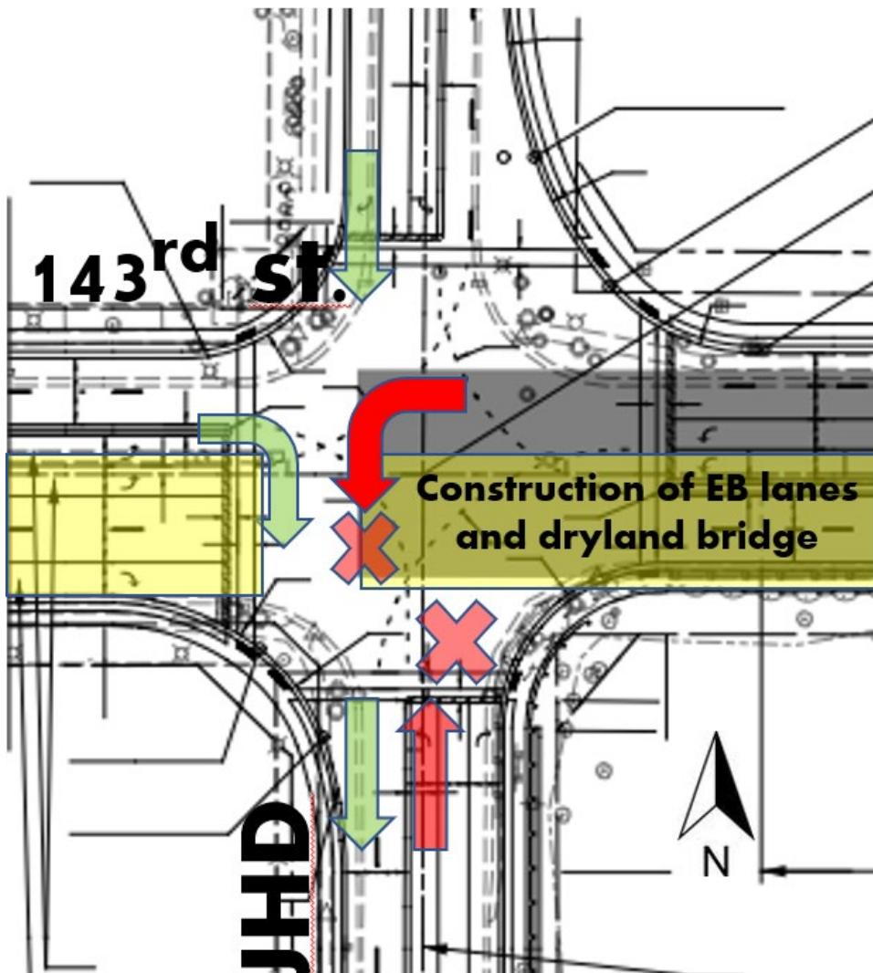
The above figures shows potential restricted movements in red arrows during construction of the eastbound lanes that would require a partial / one-way detour for NB traffic on JHD.
