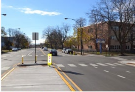
Refuge Island and Buffered Bike Lane on Vincennes Ave at Westcott School
