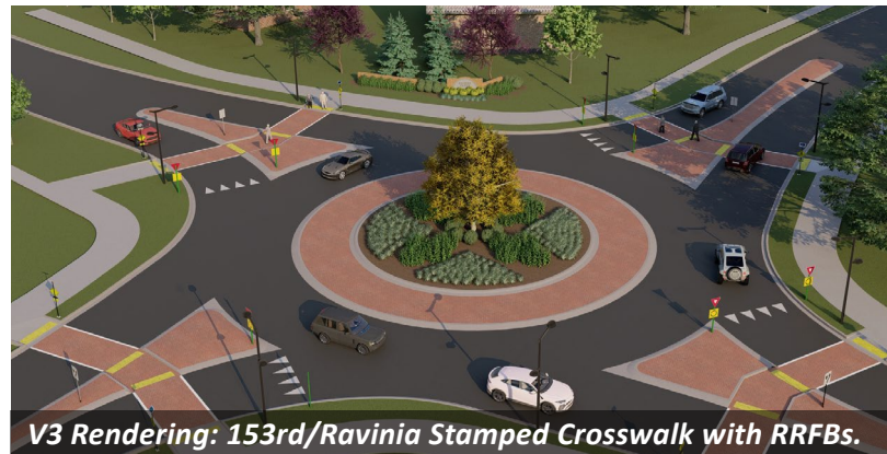
Recently designed roundabout by Strand incorporating RRFB.
