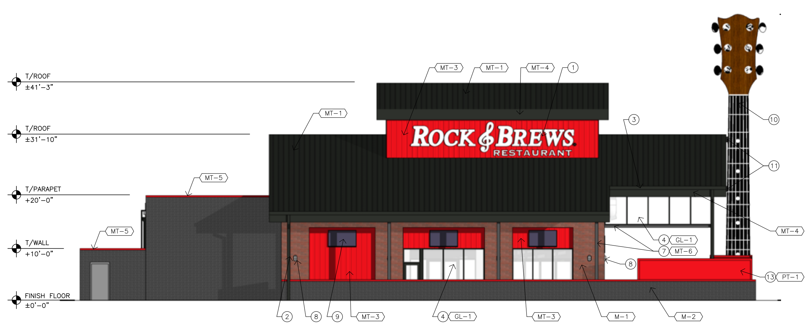
3 WEST ELEVATION SCALE: 3/32"=1'-0"
