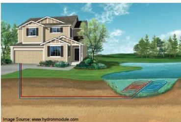
Left: Renderings that show residential and non-residential applications of hydrothermal heat pump systems using detention ponds.
