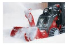
**SNOWTHROWER** Two-stage design with the power to handle the toughest snow conditions. Replaceable scraper. Adjustable skids. Overall Width: 48" Clearing width 44".
