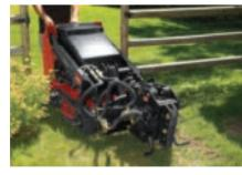
**VIBRATORY PLOW** Reduce time spent on irrigation or cable installations. The vibratory plow optimizes pipe-pulling performance while minimizing turf damage. Extremely tight turning radius allows for tight maneuvering in confined spaces.
