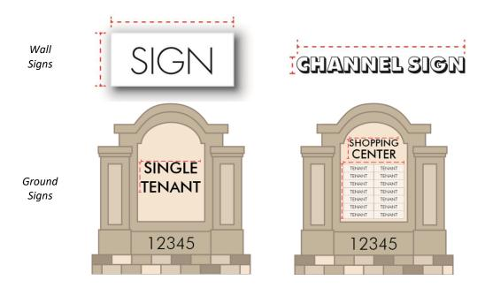
2. **Sign Height (Ground Sign).** A ground sign shall be measured vertically from the adjacent average natural grade to the top of the sign. The measurement includes the full height of the sign, including the base or support structure and any design element surrounding or enclosing the sign face.
