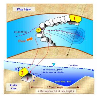
This allows sediment from upstream to deposit and shifts the thalweg away from the banks. Correct spacing of vanes will maintain or flatten the creek bed slope and reduce velocities. Soil lifts and rock toe are used to stabilize steep slopes. These natural channel design techniques will be re-evaluated to determine if they still apply under the current bank conditions.
