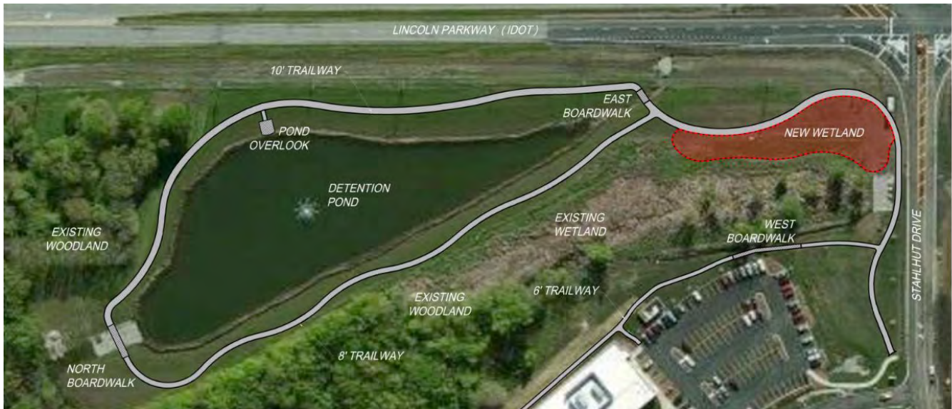
The design weaves a multi-purpose trailway around and over existing wetlands. In addition, 30 acres of new wetland was created for mitigation purposes.
