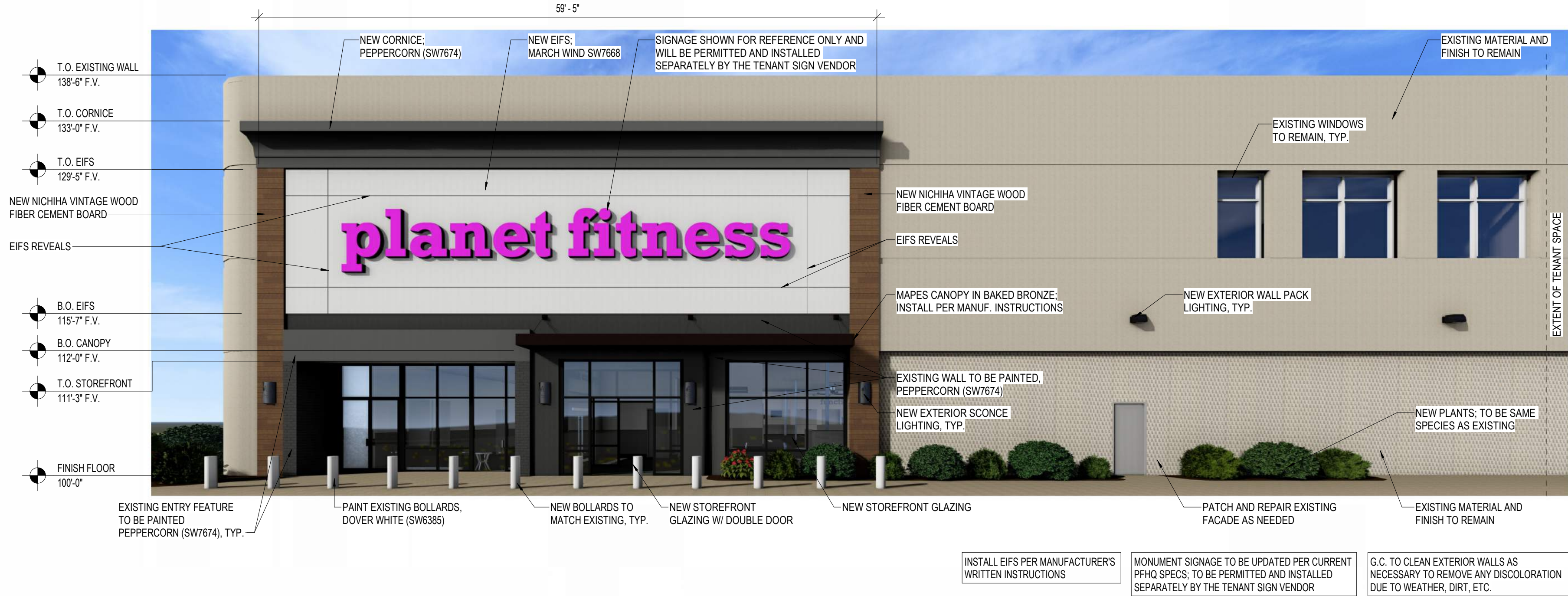
1 EAST EXTERIOR ELEVATION 1/8" = 1'-0"
