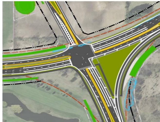
Proposed intersection with added fourth leg, raised medians, dual left-turn lanes, right-turn bypass lane, and modernized signals.
