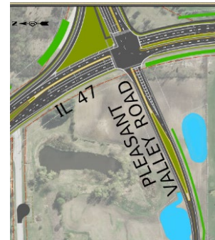
Realigning Pleasant Valley Road for a quarter mile, creating a fourth leg at the intersection with IL 47 and IL 176.
