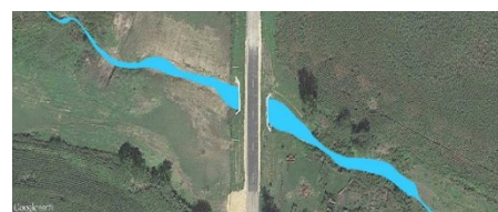
Before and after aeriels of Kent Road culvert – natural stream migration after culvert location was shifted.
