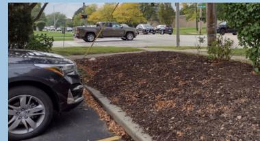
**The existing parking lot is deceptively lower than the adjacent sidewalk, likely requiring additional grading or a retaining wall to limit parking impacts.**
