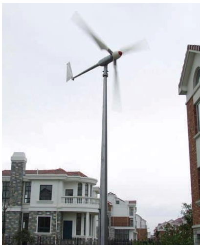
Figure 5: Example of a freestanding MINIWECS monopole turbine
