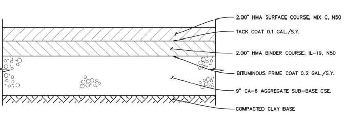
BITUMINOUS PAVEMENT DETAIL
