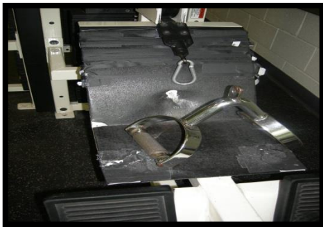
Duck taped, cracked and damaged
