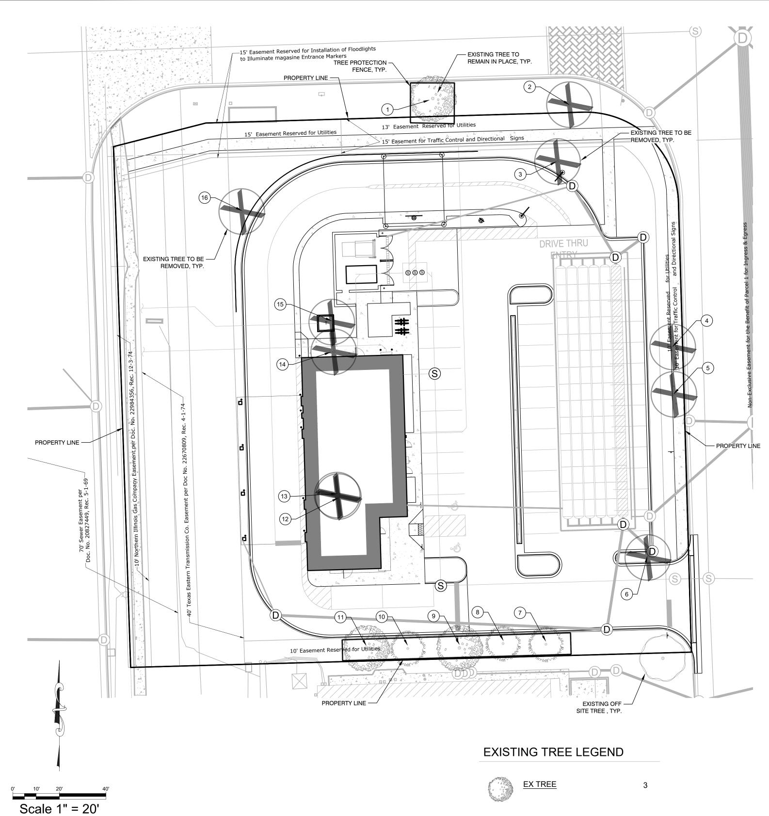
NOTE: TREE PROTECTION FOR ANY PRESERVED OR RELOCATED TREES MUST BE PROVIDED PER DETAILS AND SPECIFICATIONS ON SHEET TD-2. THESE MUST BE UP PRIOR TO THE COMMENCEMENT OF ANY WORK AND MAINTAINED THROUGHOUT CONSTRUCTION.
