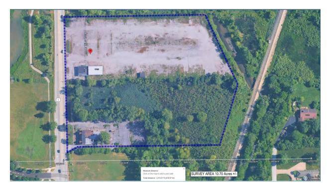
The areas to be topographically surveyed (Survey Area) shall include the aforementioned property and shall extend <u>25</u> feet beyond the property lines and to the <u>centerline</u> of adjoining roads or streets.
