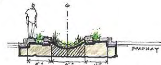
Detail 2 - Cross section showing a narrow section of the median with one bioswale
