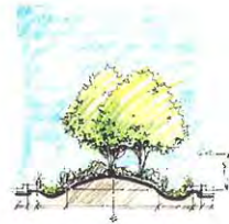
Detail 1 - Cross section showing a wide section of the median with two bioswales
