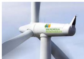
Far Left: WECS signage that identifies manufacturer in a small area per code requirements.
