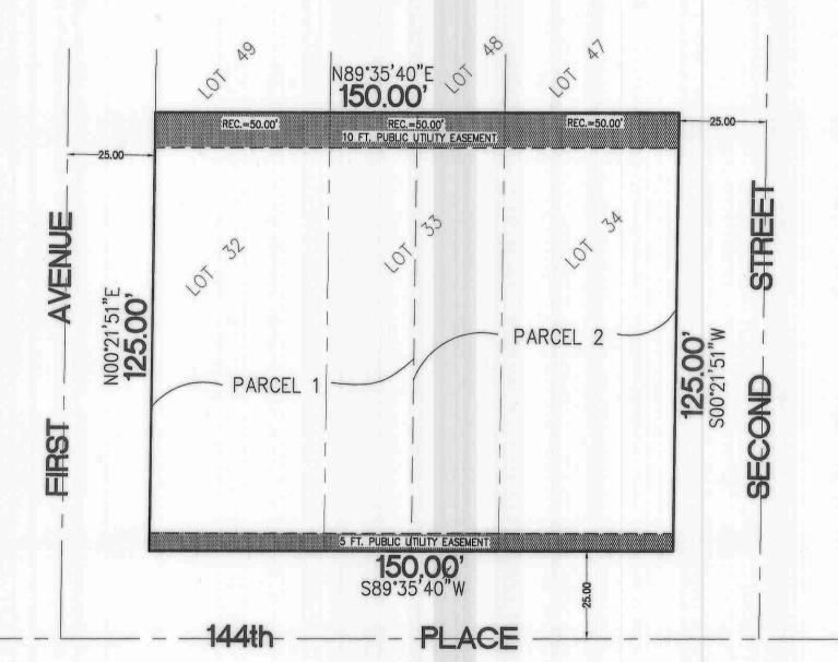
N'LY = NORTHERLY S'LY = SOUTHERLY CH = CHORD LENGTH E'LY = EASTERLY (r) = RECORD VALUE WLY = WESTERLY (m) = MEASURED VALUE TYP = TYPICAL P.U.D. = PUBLIC UTILITY & DRAINAGE EASEMENT
