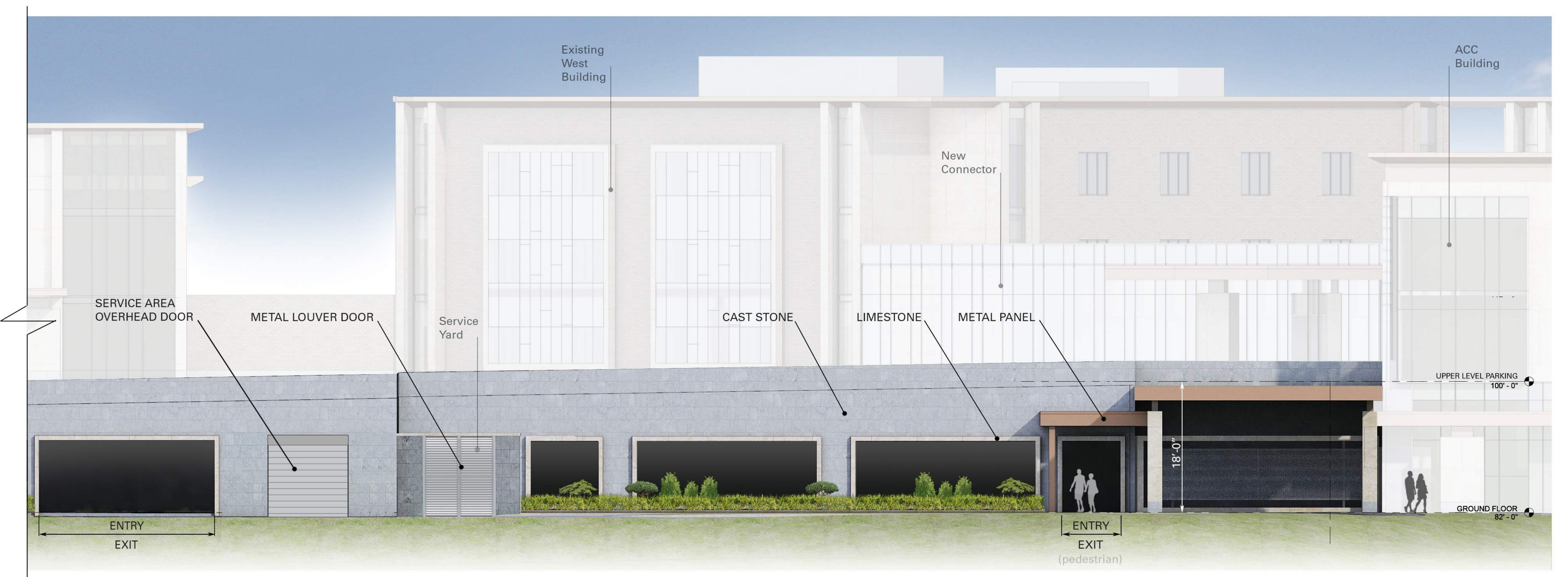
EAST ELEVATION OF PARKING DECK SCALE: 1/8" = 1'-0"
