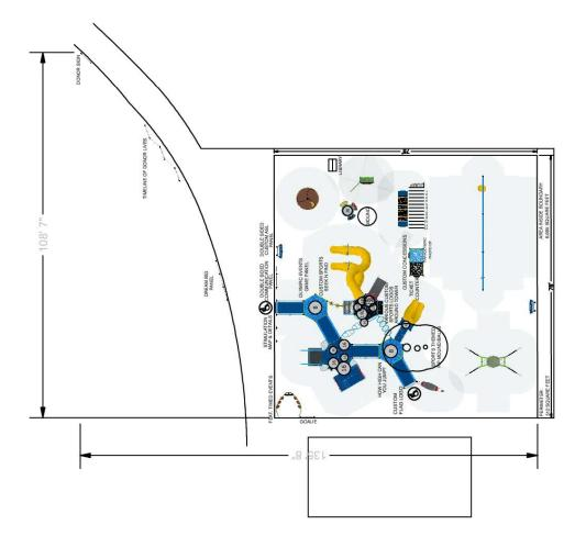
The use and layout of play components identified in this plan conform to the CPSC guidelines. U.S. CPSC recommends the separation of age groups in playground layouts.
