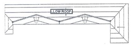
1/8" PER FOOT TAPERED POLYISOCYANURATE INSULATION WITH 1/4" PER FOOT SADDLES
