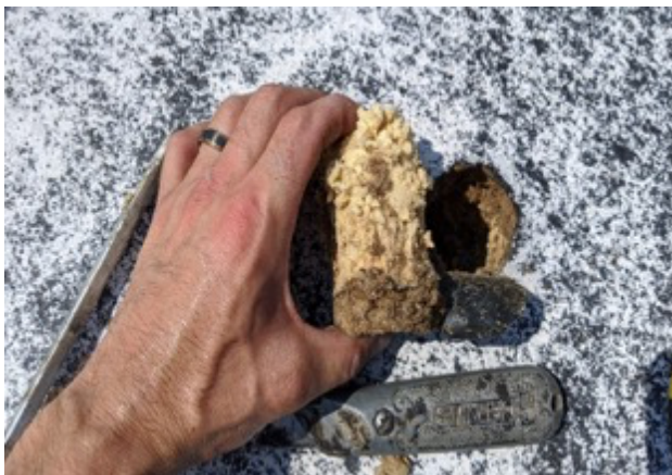
Core sample- 2.5" Iso, .5" Wood fiber cover board
