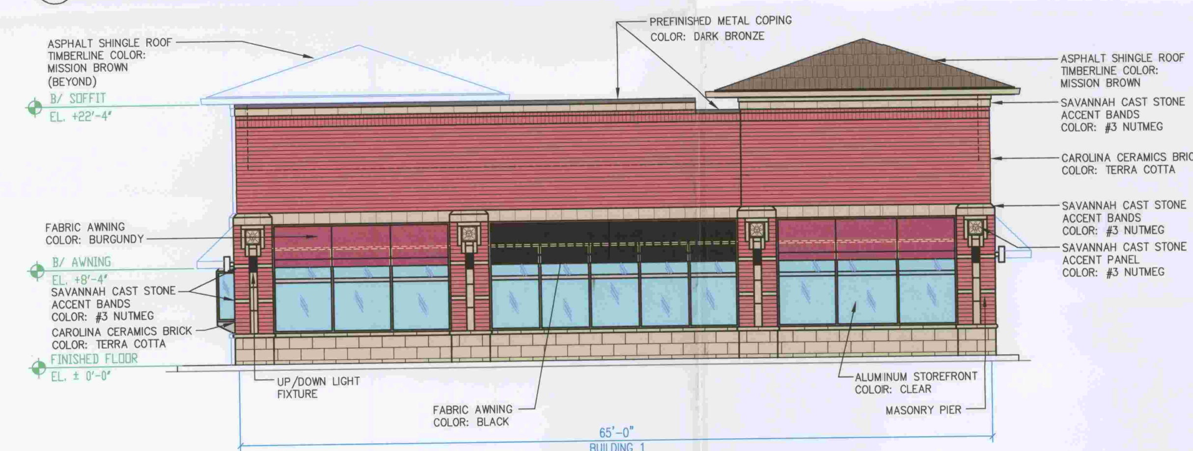
3 BUILDING 1 - SOUTH WALL ELEVATION
