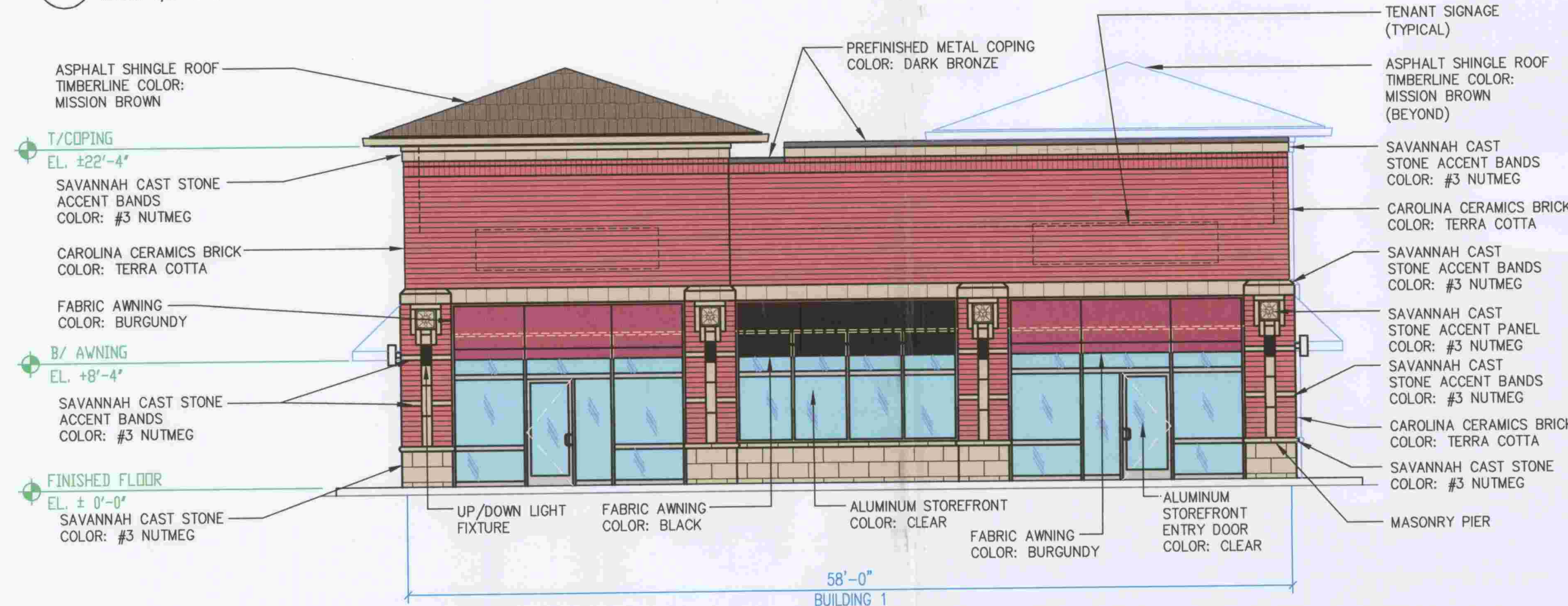
2 BUILDING 1 - EAST WALL ELEVATION
