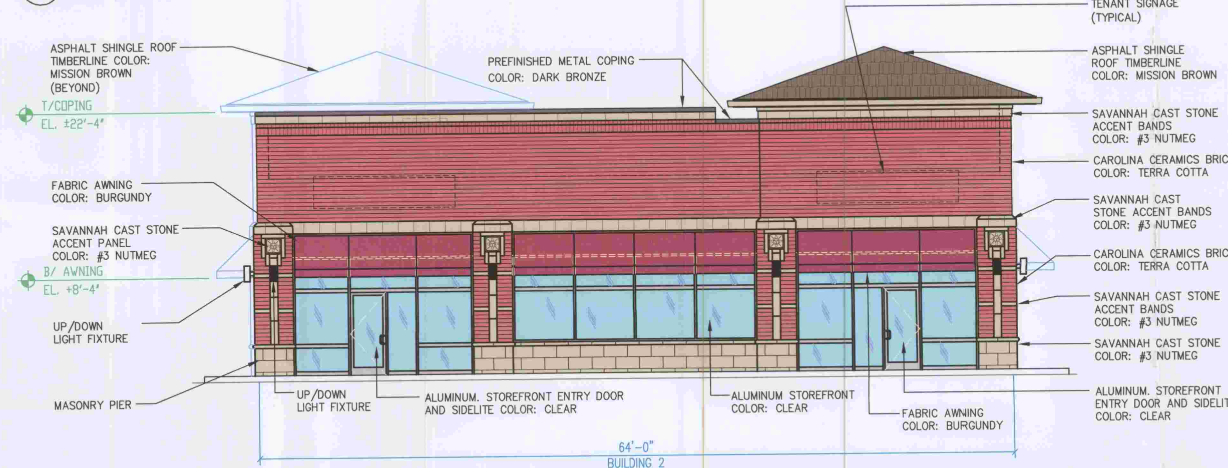
6 BUILDING 2 - EAST WALL ELEVATION
