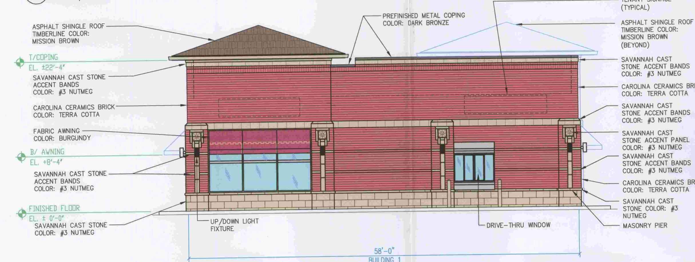
4 BUILDING 1 - WEST WALL ELEVATION
