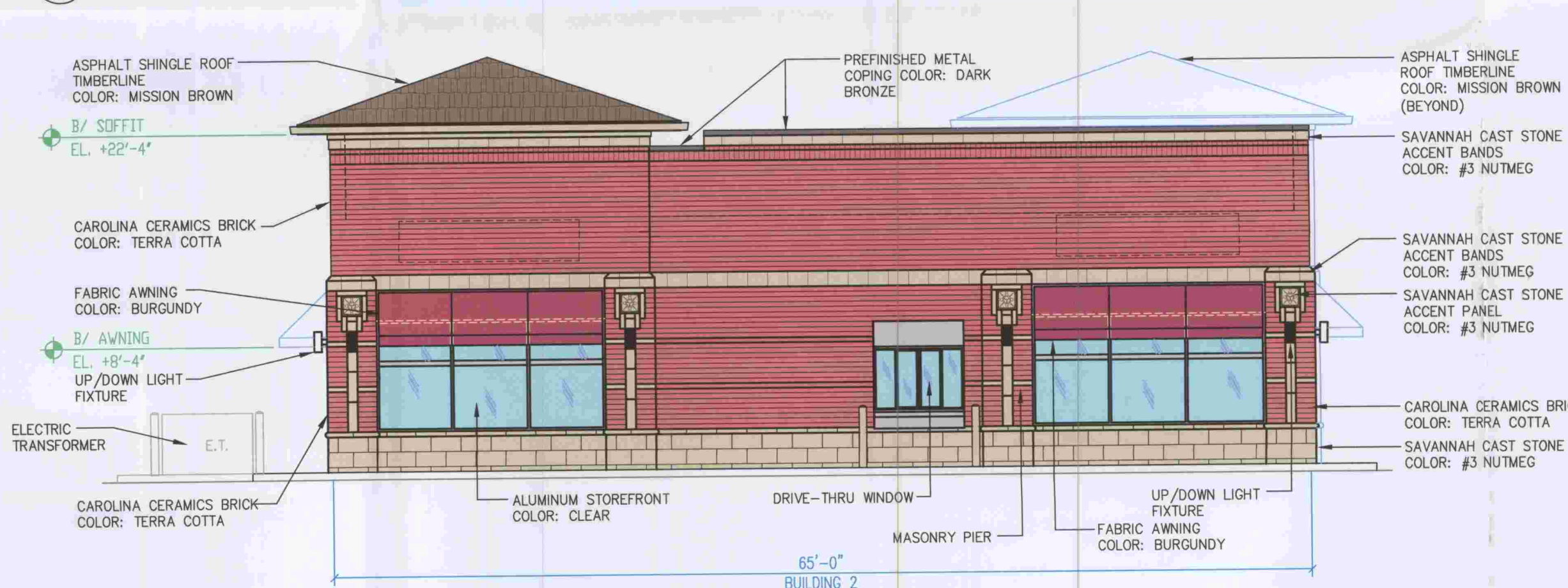
7 BUILDING 2 - SOUTH WALL ELEVATION
