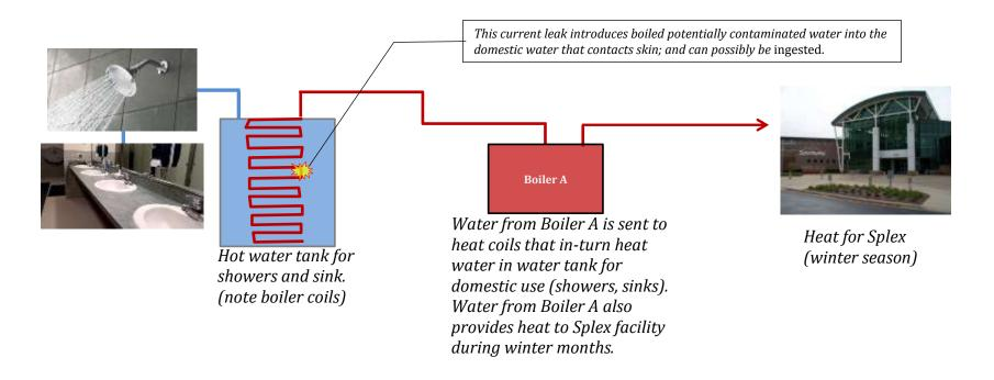
The replacement of this "heater coil bundle" would cost upwards of \$10,000. The Spelx Domestic Water Project, which would remove the hot water tank and replace it with a boiler, is scheduled to be initiated in FY17. It may be prudent to forego putting good money into this bad tank and request for CTS to provide a quote for what it would cost to accelerate the removal/replacement of the hot water tank only.
