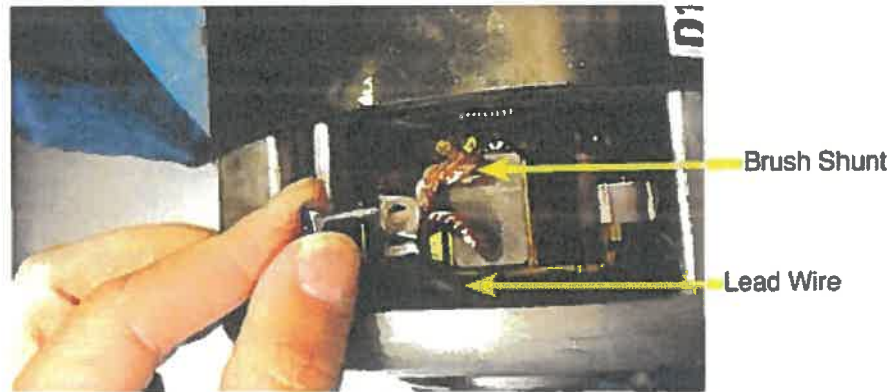
Figure 29 Replacing Brush Shunt Bolt
